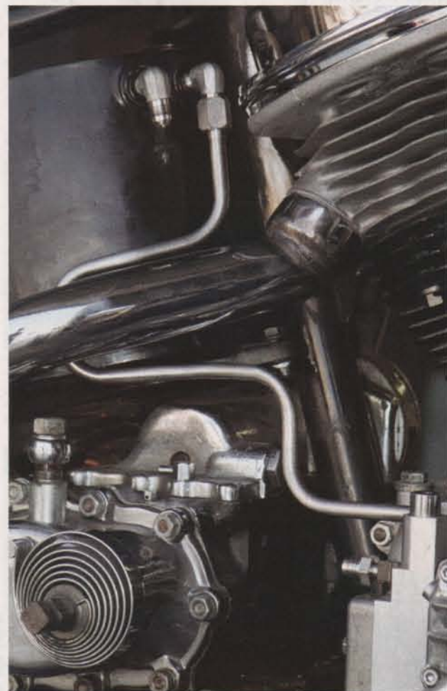
Mark's first step was to install aircraft-grade, 90-degree, -4 AN to 3/8 NPT elbow fittings in the oil tank and straight -4 AN to 3/8 NPT in the oil pump. The AN type of fitting uses a 37-degree flare; it is standard in the aircraft industry.
