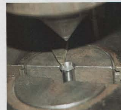
Once the tubing has been formed, a flare nut is slipped over the end and the tube is inserted into a flare-forming die in a Conrac flaring machine. This machine puts a precision flare on the end of the tube.
