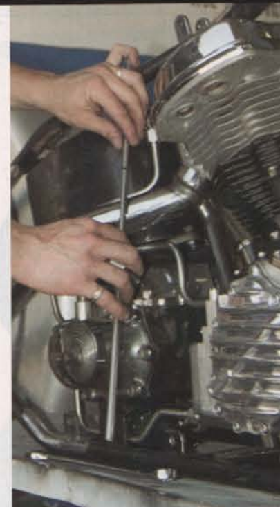
Comparing this tube to the vent tube he had installed previously, he eyeballed the amount of bend he would need.
