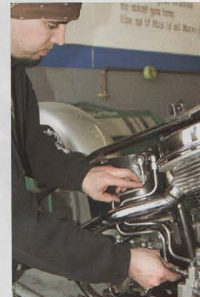
Once Mark has the tube finished, he fits both ends to each of their corresponding fittings before threading the flare nuts on. This way there is no stress or binding on the line.
