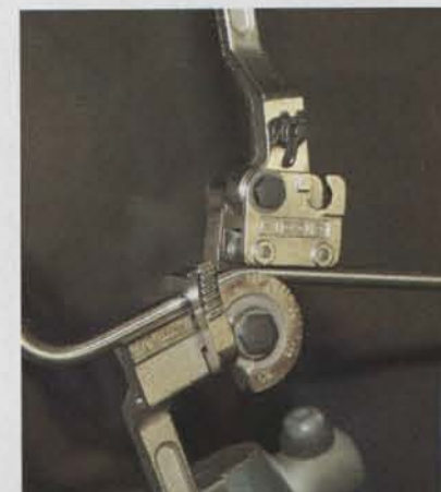
Mark's second bend is to position the tube next to the oil tank while keeping it behind the exhaust pipe. Knowing just where to bend the tubing and how much to bend it, comes from a lot of experience.
