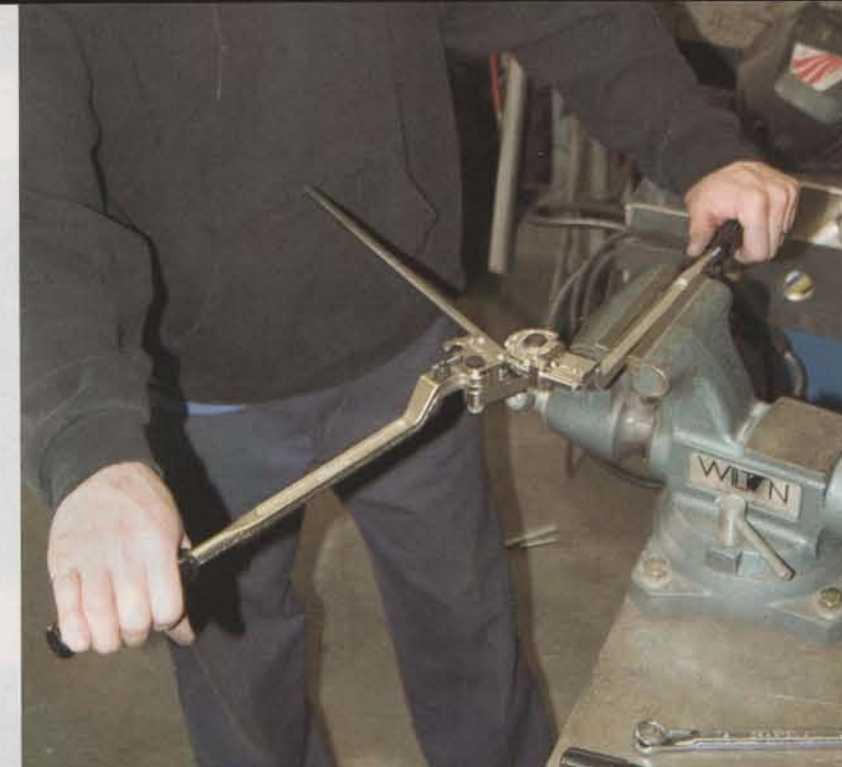
He uses a high-quality mandrel-type tube bender to keep from kinking the tubing.
